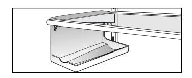
The **Tilt Out Refrigerator Door Bins** (select models) are ideal for storing awkward containers such as liter bottles and bagged items. By tilting the bins outward, space is opened up to conveniently load or retrieve contents.
